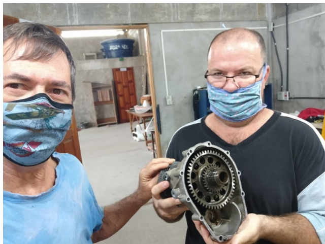
Here is the reduction gearbox we sent in today for inspection.
